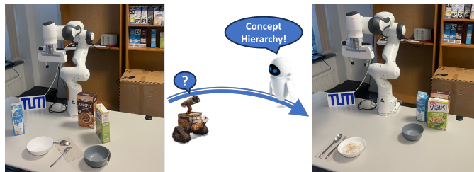
Fig. 1: “How to transform the left environment into the right one?” The knowledge in the Concept Hierarchy enables household robots to represent environments and to create a plan to execute tasks.
