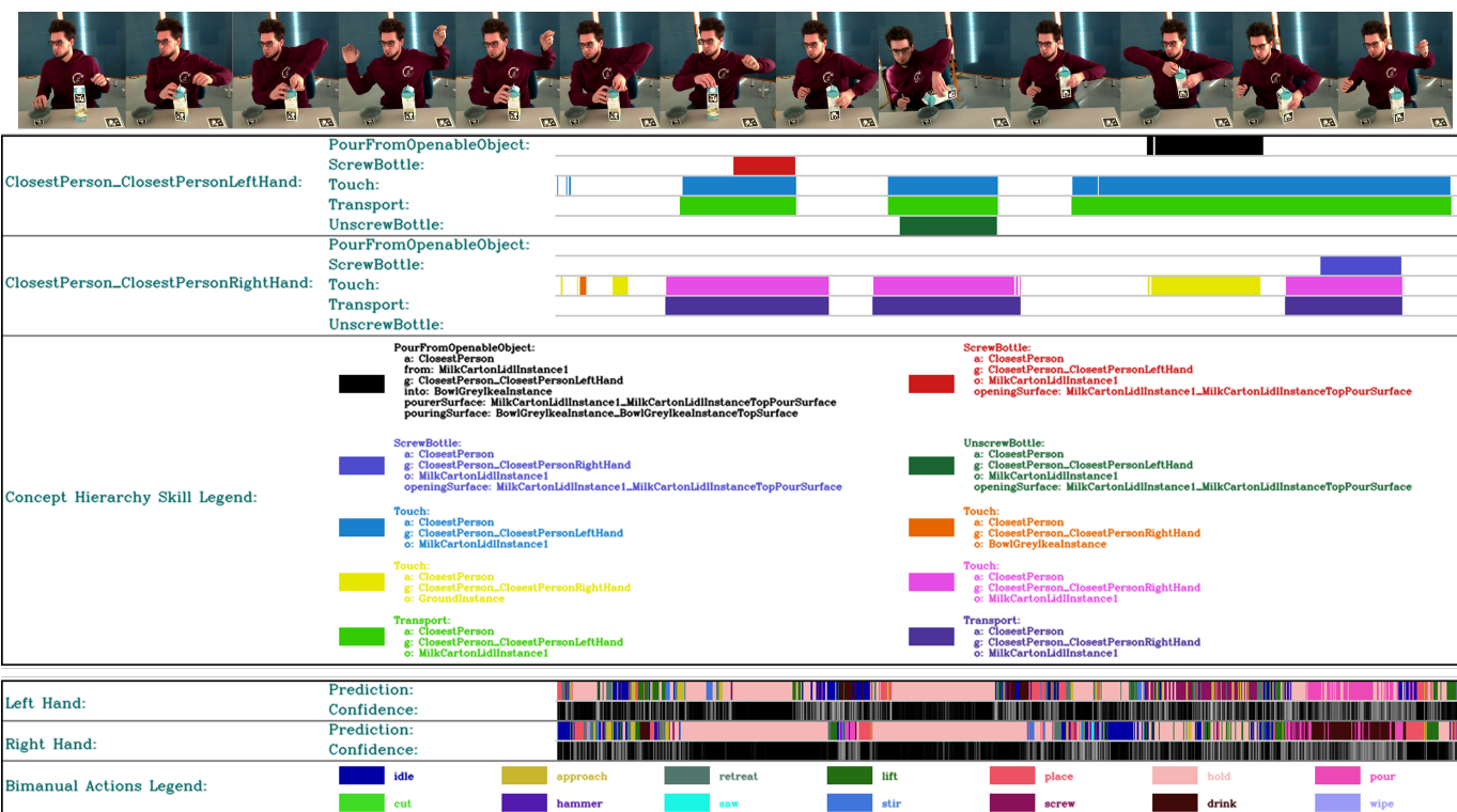
Fig. 4: Skill recognition result of a bimanual task of pouring milk into a bowl. The demonstration is composed of closing and then opening a milk box with the left hand, pouring milk into the bowl, and closing the milk box with the right hand. The upper figure presents the Skill instances our method recognizes for each hand and Skill type. The colors help distinguish Skills of the same type with different parameters. The lower figure shows the results of [9] that was trained on the Bimanual Actions dataset [10] (darker confidence = higher softmax output).
